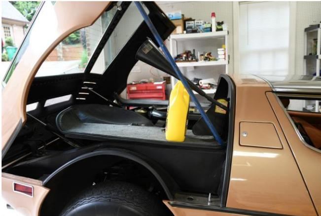
Funnel with hose to refill the cooling system
