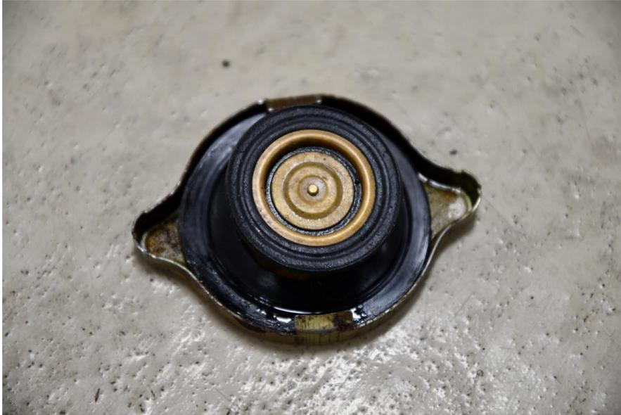
You do not want air to come into the expansion tank once an overflow tank is installed, therefore make sure the radiator cap has a rubber seal along the top of the cap.
