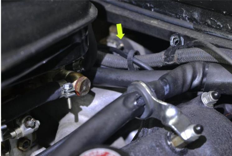
Disconnect small hose on top of thermostat housing to permit air to escape.
