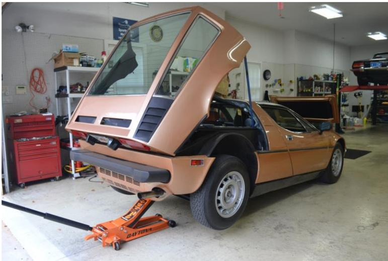
Lift the rear of the car when draining and refilling the cooling system.
