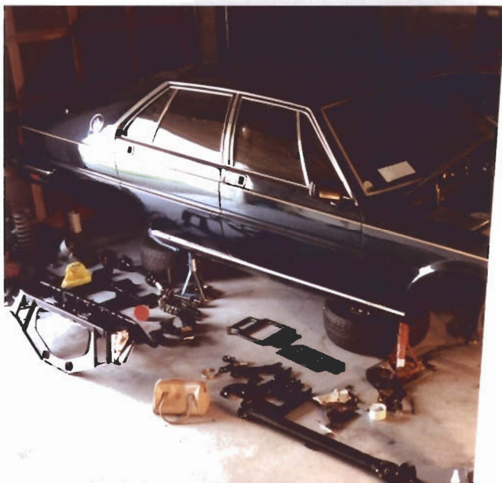
At one point of the restoration you can see all the parts off the car. Note the rear transaxle frame, drive shaft, A-Arms, and wife's purse to pay for everything!
