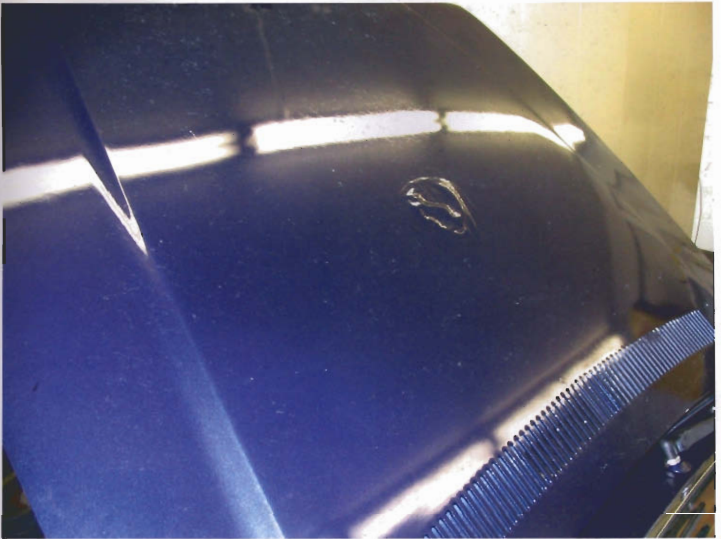
The large bubble on the hood from the heat.
